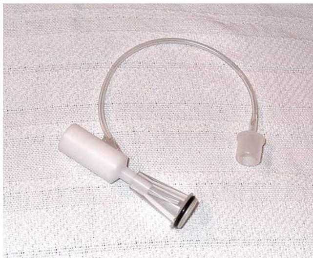
Figure 1. Patient breathing circuit used for rodent anesthesia
