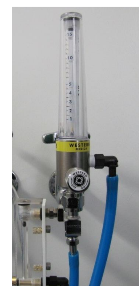
3. View of regulator on the vacuum outlet. The vacuum flow rate must be carefully set or the SCOOP may fail to scavenge all the anesthetic gas, or may pull the gas so fast that the animal is not properly anesthetized.
